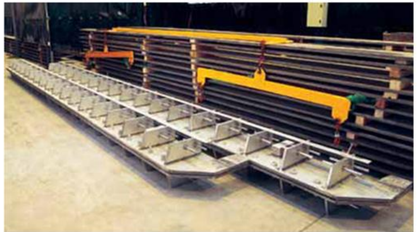
Road Deck Endplates. Project: Dartford East Tunnel, UK (Contractor: Kvaerner/Skanska)
