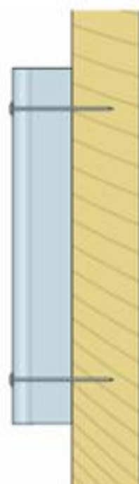
Channel Nailed to Formwork
