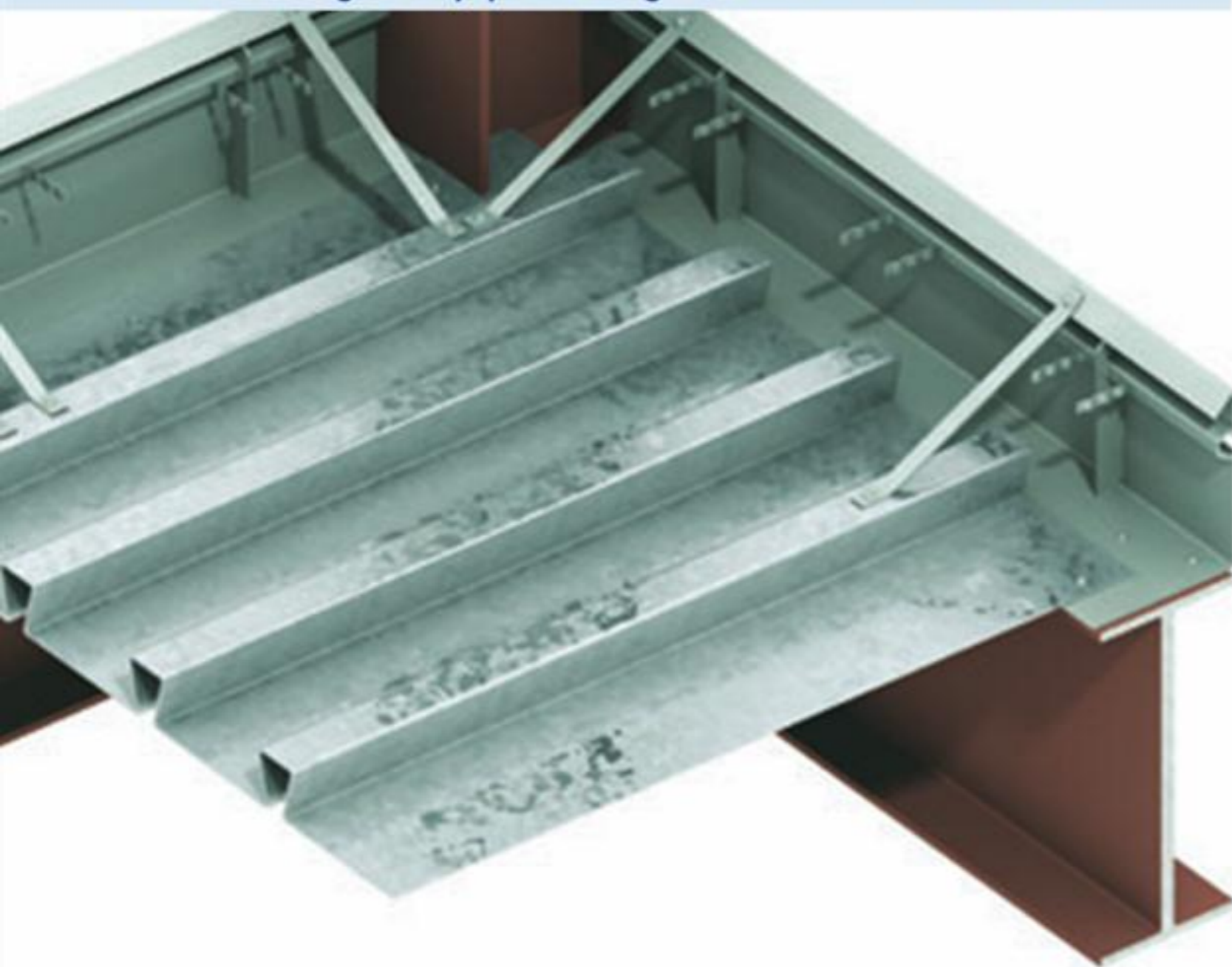
Corner Detail Showing Fixing Straps Between CombiDeck and Metal Deck Shuttering
