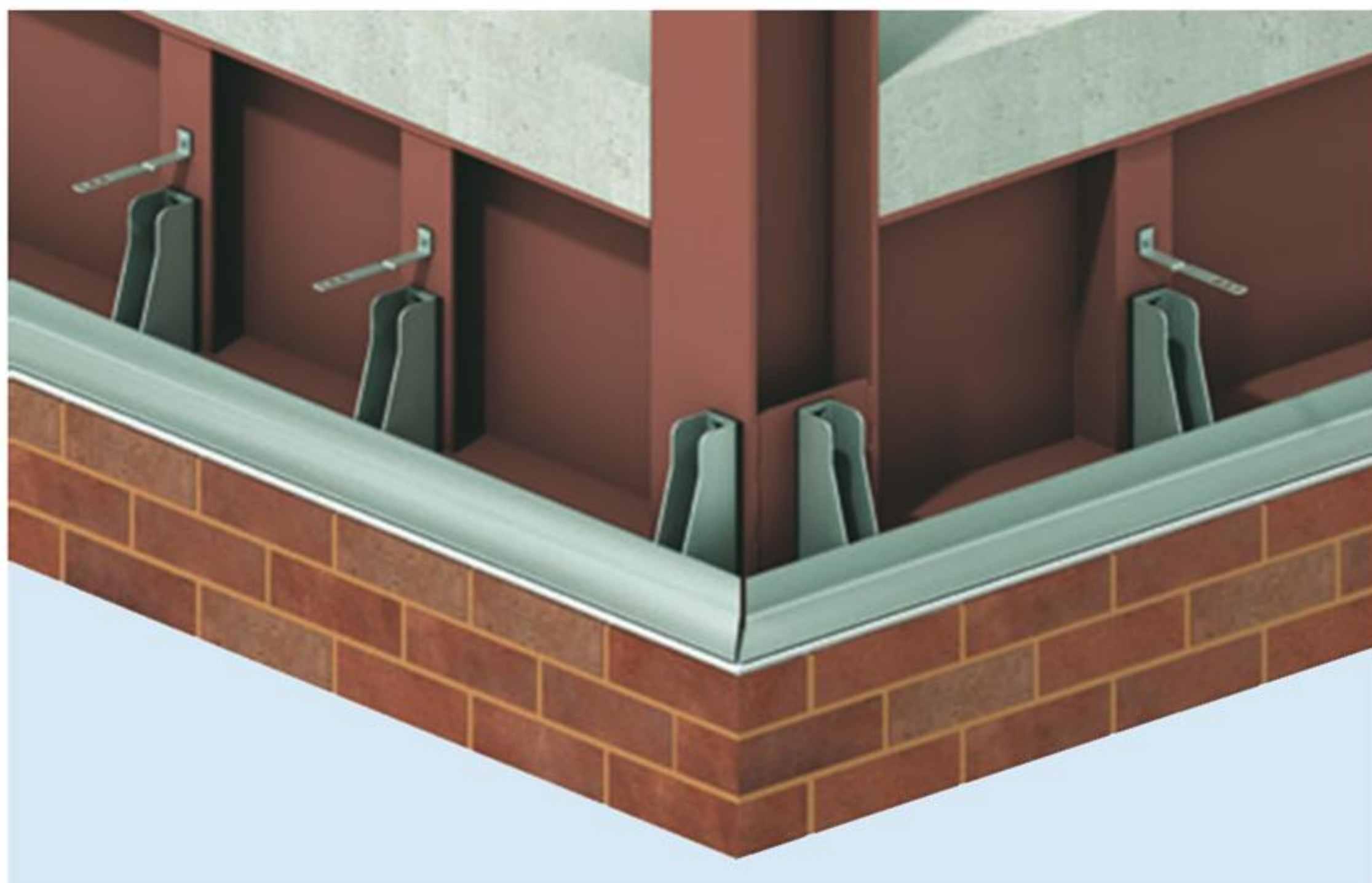
MDC Support System Bolted to Steel Edge Beam Stiffeners and a Corner Column
