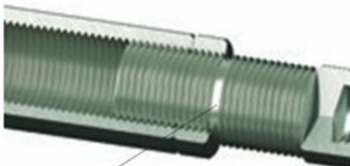
Groove is protruding from locknut
