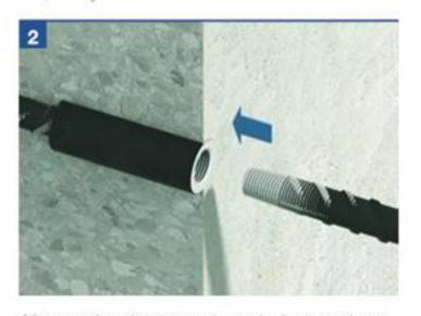
After casting the concrete and when ready to extend, remove the plastic end cap (and nailing plate where appropriate) from the coupler. Position the continuation bar in the
