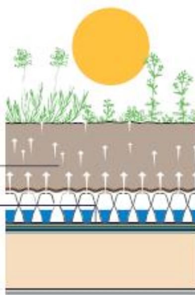
Fig 9: How a green roof releases moisture
