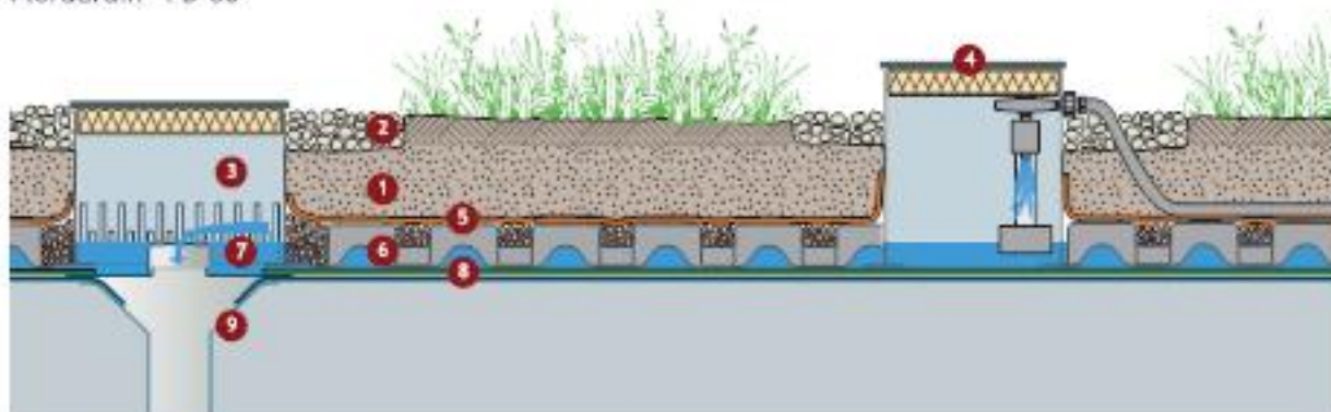
Fig 31: ZinCo Irrigation System
