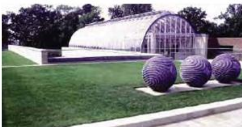
Lawned intensive green roof with Floradrain® FD 60 drainage layer
