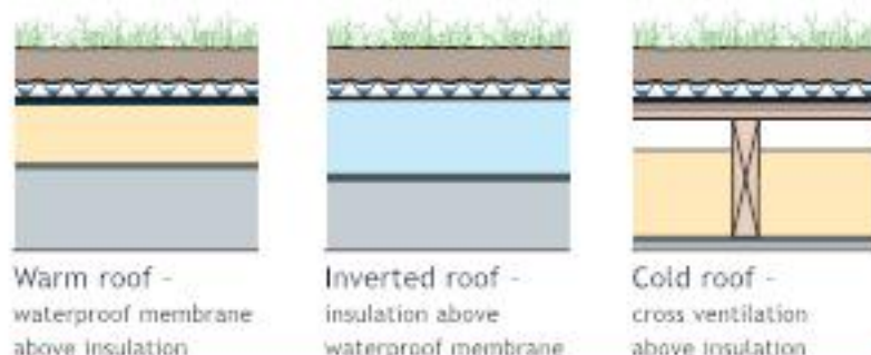
Fig 11: Roof types
