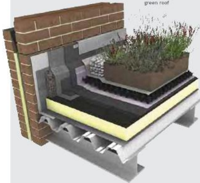
Fig 6: Semi-intensive green roof
