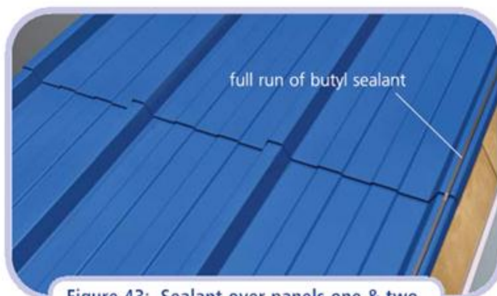
Figure 43: Sealant over panels one & two
