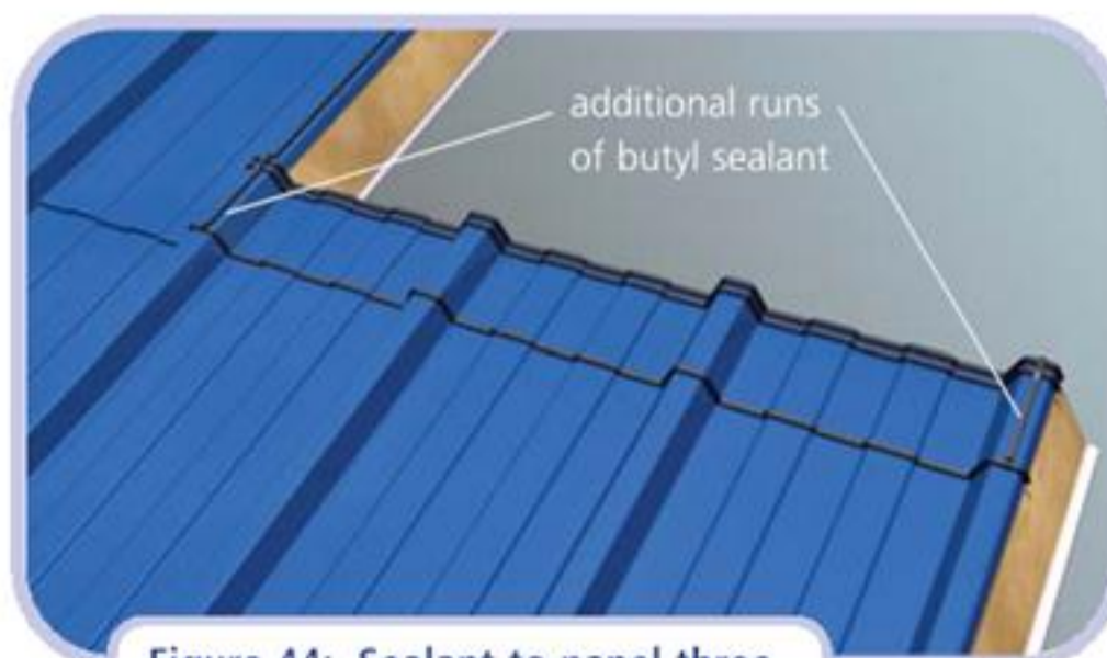
Figure 44: Sealant to panel three
