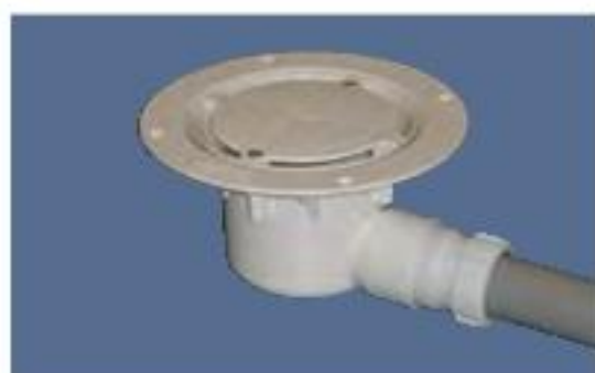
Connecting to 43mm (1 1/2") Polypropylene. Use 50mm to 43mm (1 1/2") proprietary solvent cement/compression reducer.
