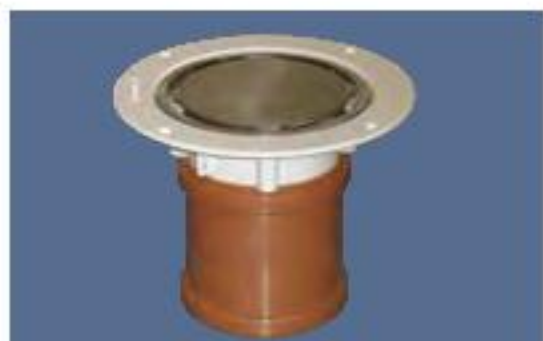
Connecting to 110mm HDPE/PVC-U (Vertical Drain Body only). Use ring seal pipe socket.
