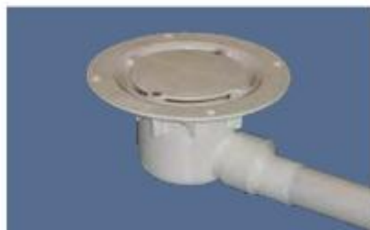
Connecting to 43mm (1 1/2") ABS. Use 50mm (2") to 43mm (1 1/2") solvent cement reducer (provided).
