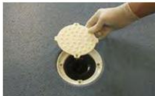
Lift aside cap taking care not to lose screws. Do not remove Clamp.
