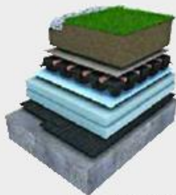
Inverted green roof, traditional torch-on
