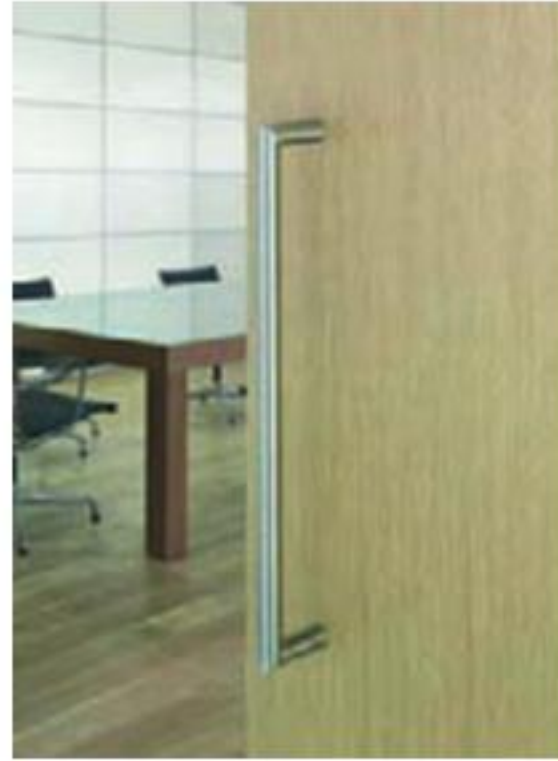
1770 Modric pull handle with bolt through fixings. 400mm centres. Finishes: SS • PS
