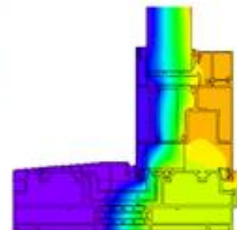
Distribution of isotherms in the MB-77HS HI window
